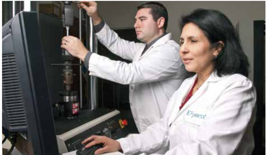
Setting up a biomaterials test on a Bionix Table Top load frame
